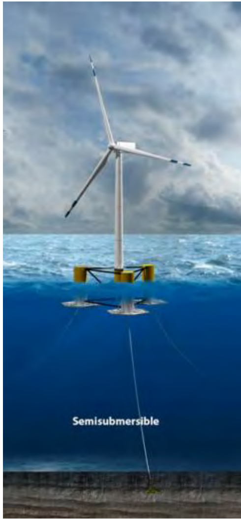
Generic Semi-submersible floating platform
